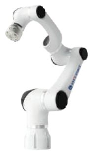
Positive pressure explosion-proof robots -proof demonstrator
