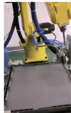
Gluing of control cabinet doors
