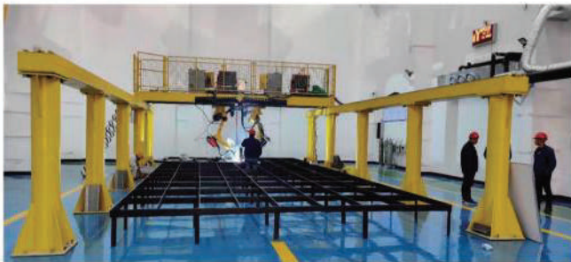
Ship Welding with Dual-robot Collaborative Laser Tracking
