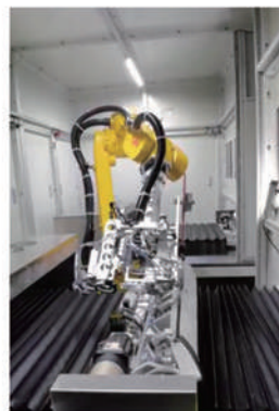
Gluing of washing machine covers
