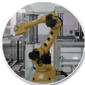
Photovoltaic basket handling
